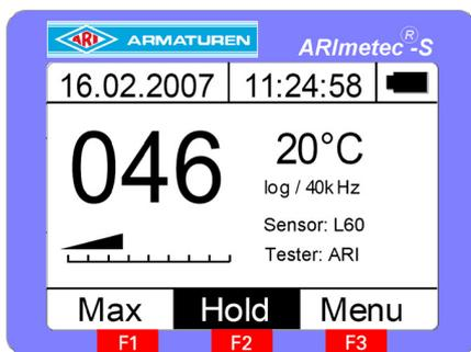
Button F2 activates the "Hold" function. This function can be used to record ultrasonic levels. It is useful, for example, if the display is not visible when the test is carried out. By pressing button "F2", you store the ultrasonic level that is measured at that instant on the display.
