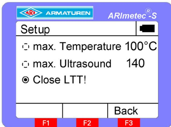
To stop recording values for the long-time test and return to check mode, you must select "Stop long-time test" in the Setup menu.
