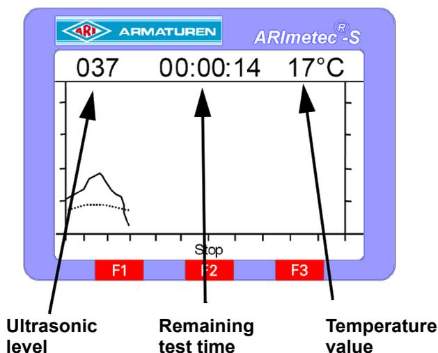
Ultrasonic levels are represented by a solid line and temperature values by a dotted line.
