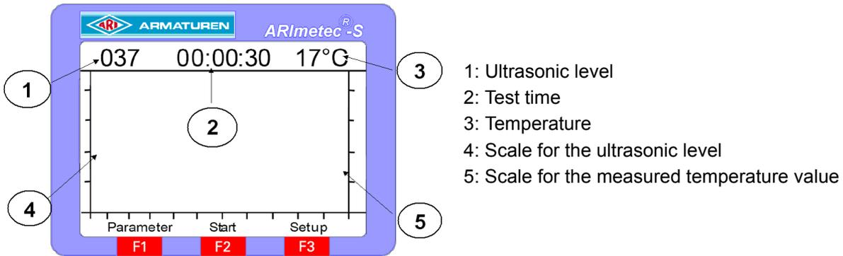
You specify the test parameters in the "Parameters" menu, which is opened by pressing button "F1". To change the display settings for the long-time test or stop the test, you must open the "Setup" menu by pressing button "F3":
