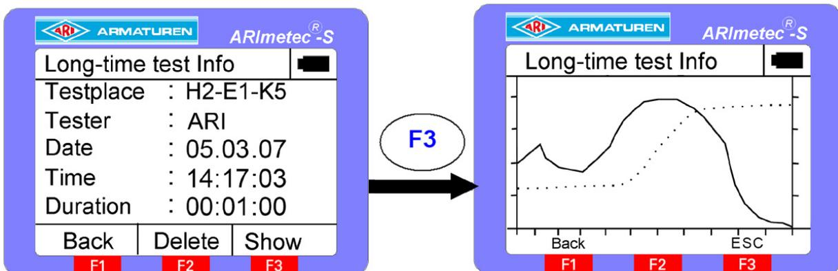
Ultrasonic levels are represented on the graph by a solid line and temperature values by a dotted line. The maximum visible time window is 60 s. If the test time is longer than 60 s, you can shift the time window by turning the control knob. The ultrasonic level is displayed on a logarithmic scale graduated from 0 to 140 or on a linear scale graduated from 0 to 240. The temperature is displayed on a scale from 0 to 800°C or from 0 to 1472°F.
