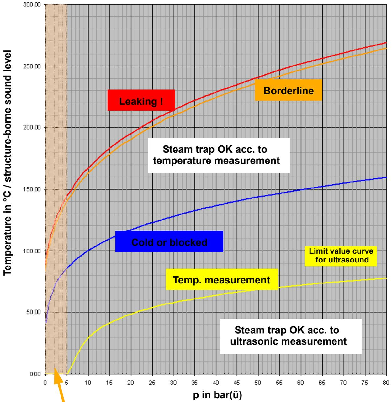
A measurement with headphones is recommended at low steam pressures in order to obtain a clear result.
