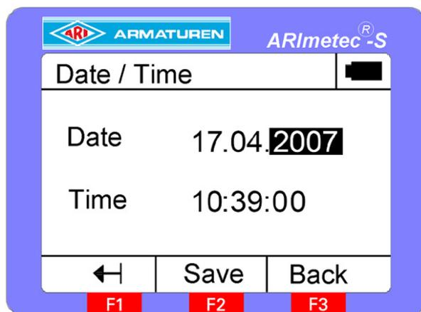
The date and time are set in this menu. You select the element you want to change by pressing the control knob and set it to the required value by turning the knob.
