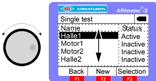
You can create a new single test by pressing button "F2", change the current test by pressing the control knob or activate the selected single test with "F3".
